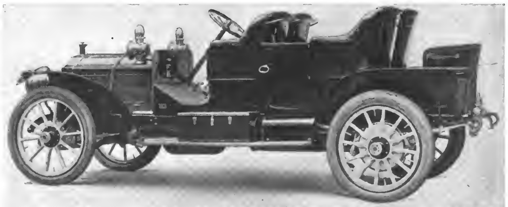
Close-coupled Body Originated by the Packard Body Department for the "Thirty" Chassis.
